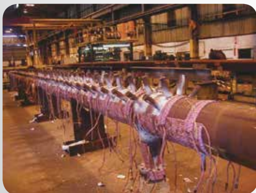
The superheater outlet manifold for the Komati power station under construction at AJT's Cape Town fabrication facility.
