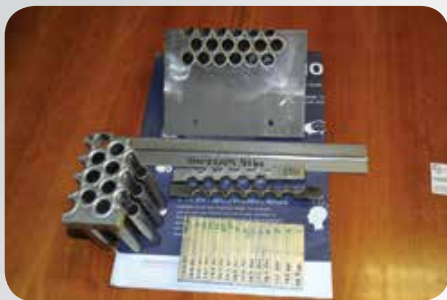
For the tar separator vessels, ND Engineering did over 140 production test plates, and were the only tendering company to achieve 100% pass rate on all of these tests.
