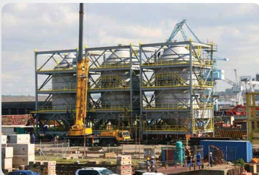
Three ammonium sulphate crystallizers for the water treatment plant awaiting shipment to Madagascar.
