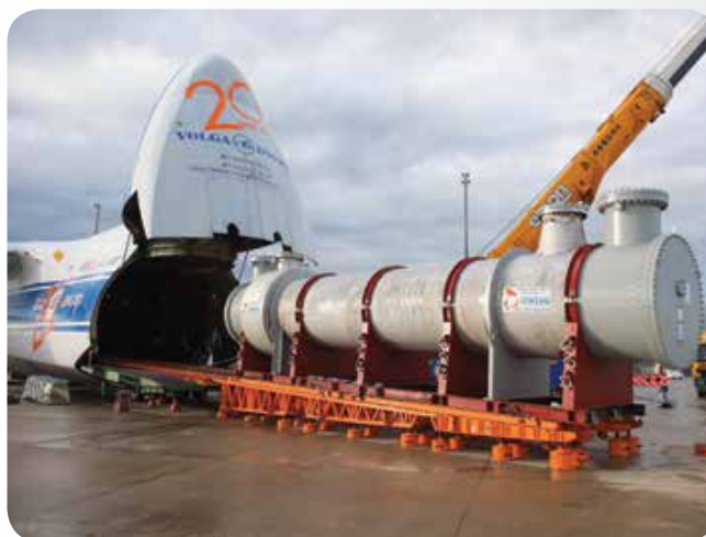
A 65 t horizontal acid cooler being airfreighted to New Caledonia.
