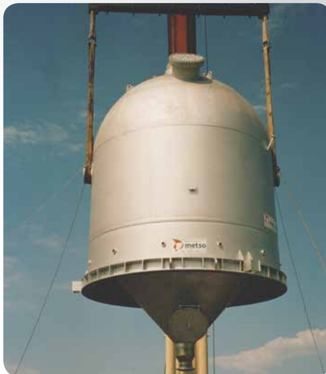
A third stage separator vessel for the recovery of catalysts in the petrochemical industry.
