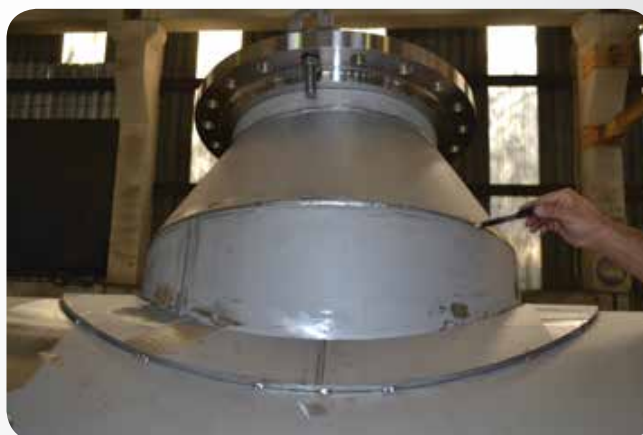
A heat exchanger vessel under construction at ND Engineering’s Queensburgh workshop.
