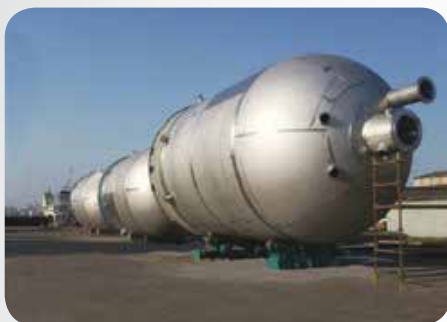
Three 285 m 3 SAF 2205 Duplex MgO Digesters manufactured for Sappi Saiccor.
