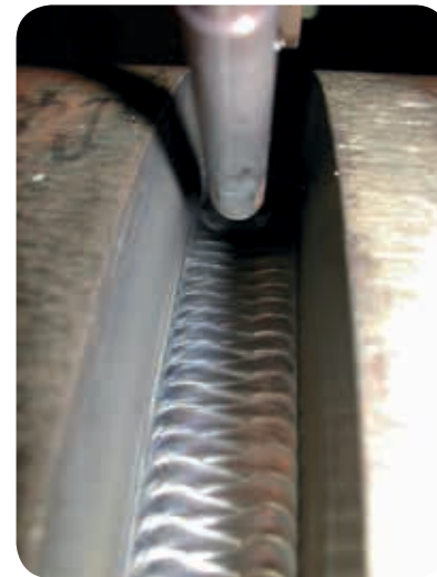
Figure 1: Zero risk/zero defects with Polysoude's mechanised and automated TIG welding technology.
