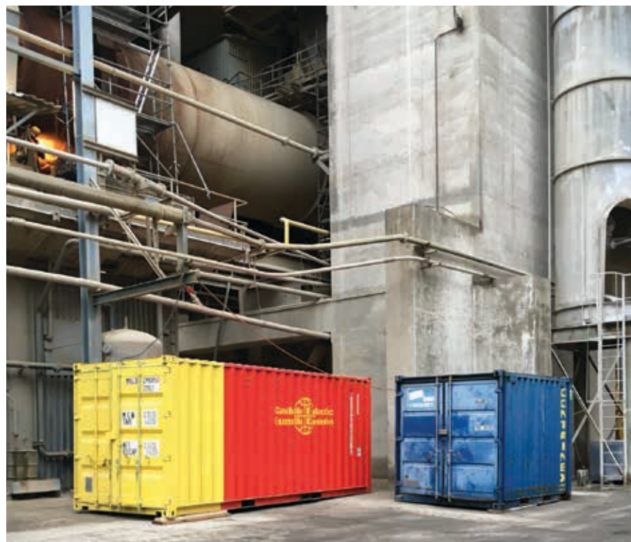
VRM repairs are done by shipping to site a fully equipped container, consisting of six mill kits, power sources, wire and control equipment.
