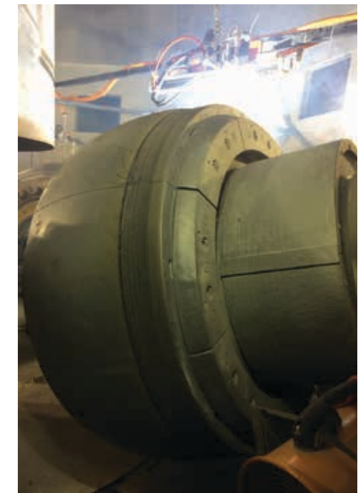
This technology enables deposition rates of up to 60 kg per hour to be achieved, which enables the entire refurbishment to be completed within three to four days.
