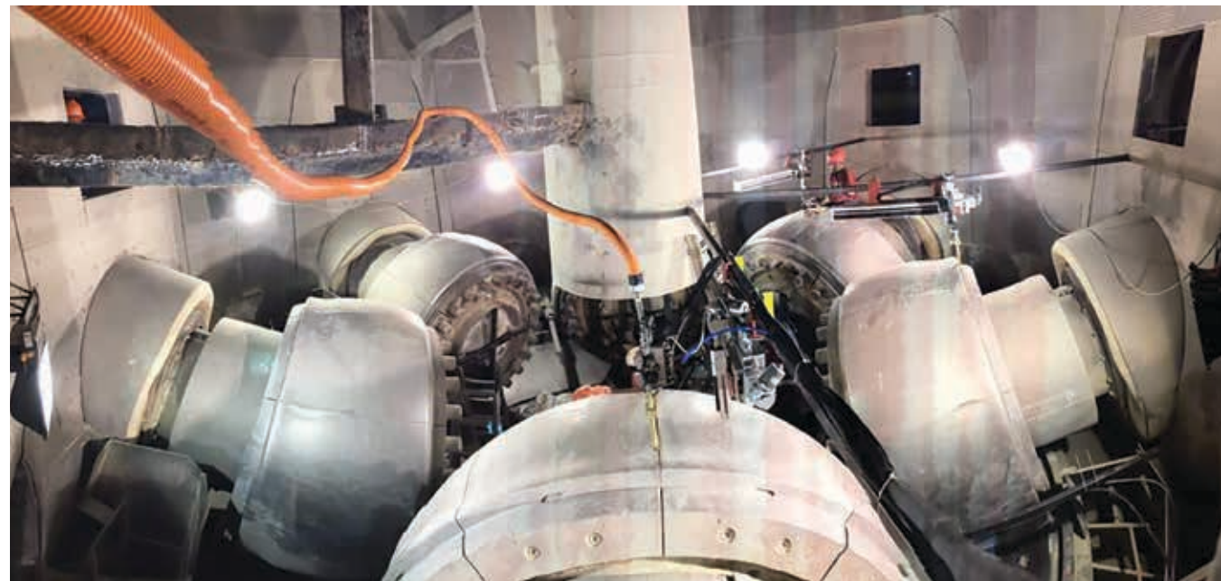
Some areas of mill media have higher wear rates and Castolin Eutectic is able to use harder wires in these areas to extend the total wear life of the mill.
