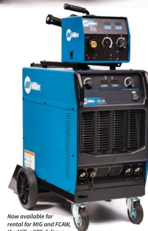
Now available for rental for MIG and FCAW, the Miller XPS delivers phenomenal output characteristics from a three-phase 380 V power source.
