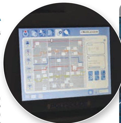
Parameters can be changed four or eight times per cycle so that they perfectly match the welding position, the penetration requirements and the prevailing heat in the pipe.
