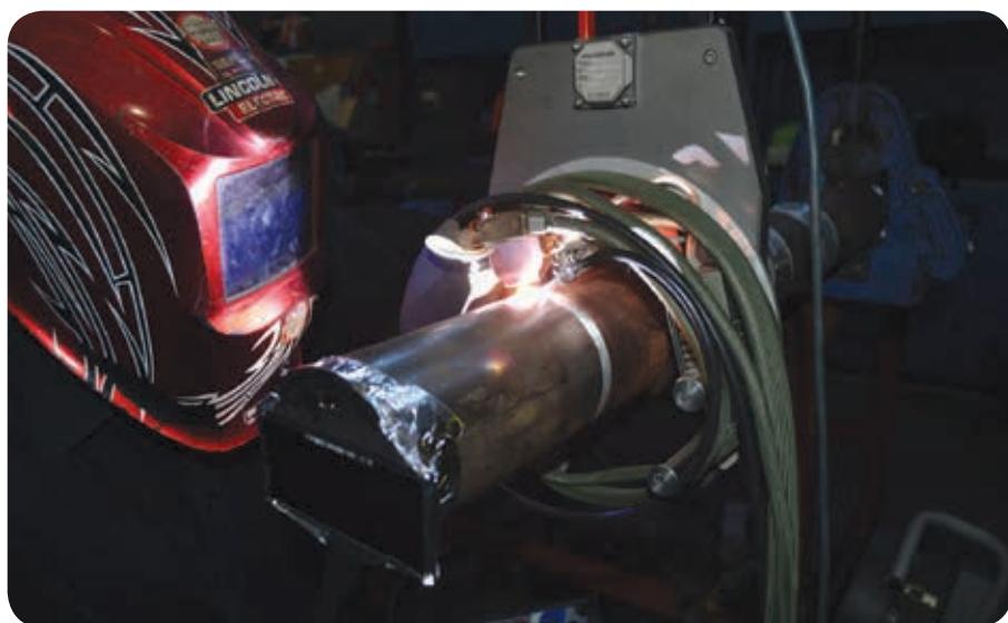
Eduan Naude demonstrates a Polysoude orbital welding solution at Renttech's Secunda premises. A TIG welding torch travels around the tubes to be joined, guided by an orbital welding head clamped onto the pipe.
