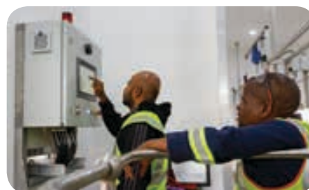
The operator attaches a manifold of cylinders to the filling station, selects the recipe required from the SCADA and the PLC will automatically fill the cylinders to the correct composition.
