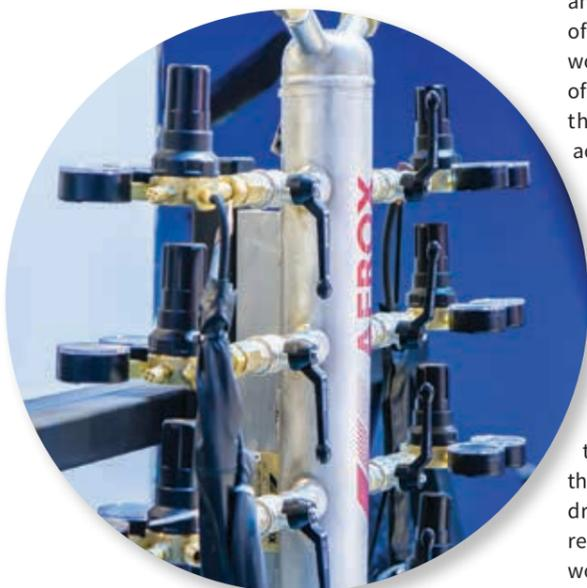
At the heart of Afrox’s 360° integrated TIG-welding solution for welding at heights is new multi-user pressure panel (MUPP), which enables up to eight TIG welders to work independently without the need for gas cylinders at the welding level.
