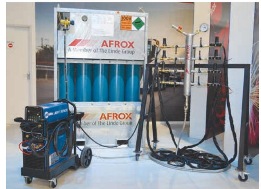
A ground supply of Argon is fed through a reinforced braided stainless steel hose to the MUPP at the welding level. Eight welders using Miller TIGRunner 280 machines can then independently control their gas flow.
