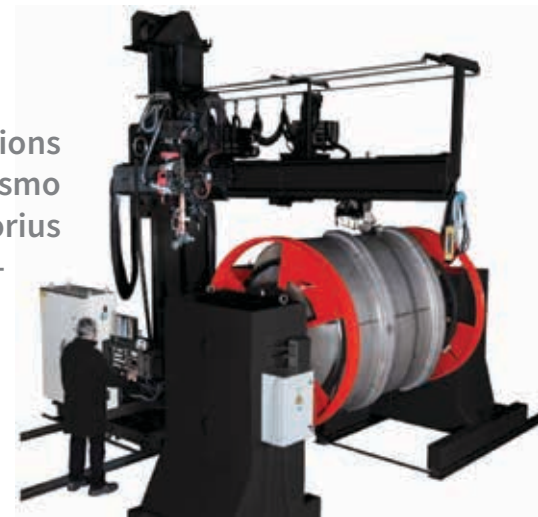
Lincoln Electric's automatic Plasma/TIG welding systems offer multiple and varied high quality seam welding solutions to suit the needs of vessel, tank and column fabricators.
