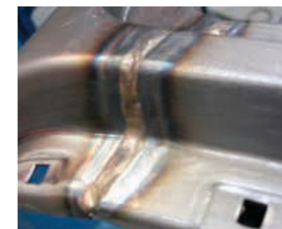
TOPTIG is ideal for robotic brazing of car body parts.
