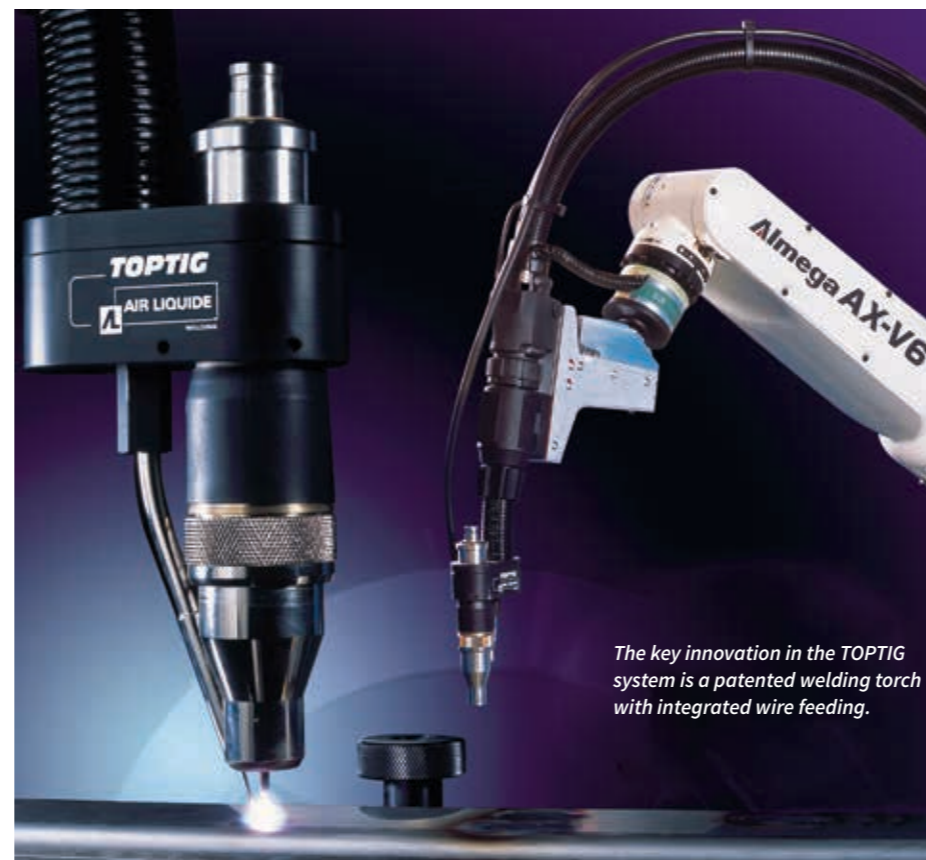
TOPTIG is ideal for robotic brazing of car body parts.
