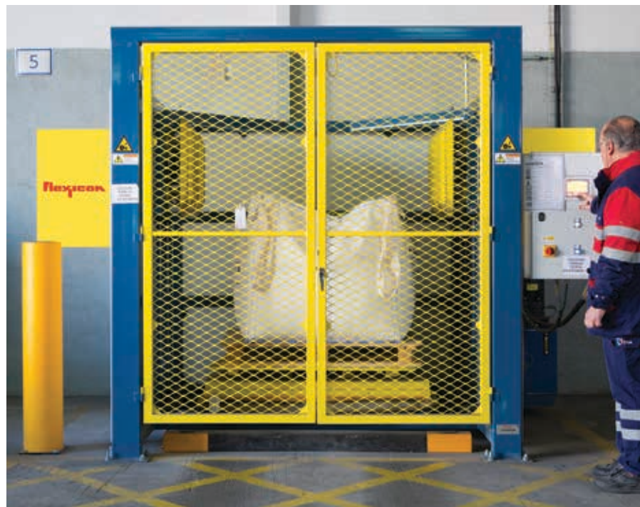
Bulk bag is loaded into the conditioner. Once the safety doors are secured, the operator initiates the conditioning cycle.
