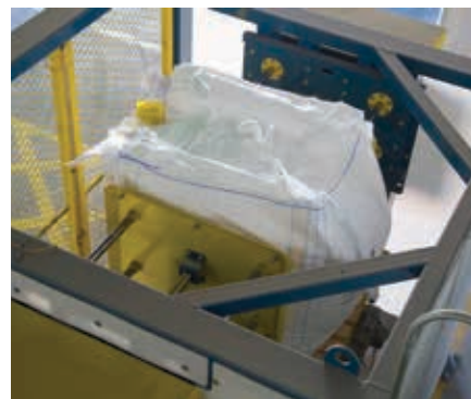
Above and below: Hydraulic rams fitted with specially contoured end plates press opposite sides of the bag to loosen solidified powders. The turntable and bag rotate 90° to condition all sides, while the scissor lift allows conditioning at all heights.
