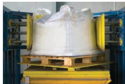
Above and below: Hydraulic rams fitted with specially contoured end plates press opposite sides of the bag to loosen solidified powders. The turntable and bag rotate 90° to condition all sides, while the scissor lift allows conditioning at all heights.
