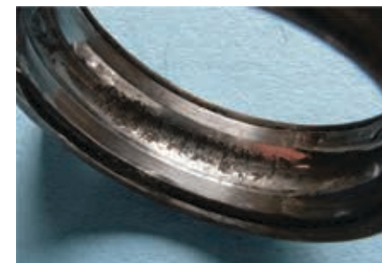
Figure 4: Rolling contact fatigue in a bearing leading to spalling of the raceway.
