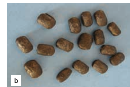
Figure 5: a) Inner race from a high speed bearing after bearing after lubricant failure; b) Rolling elements from a high-speed lubrication failure showing melted cage debris.
