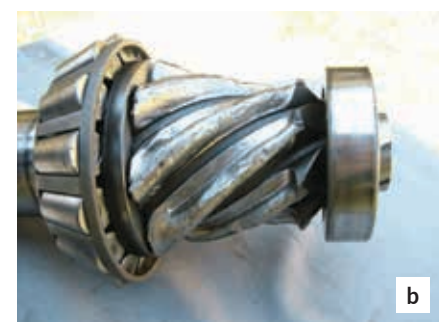
Figure 1: Both the crown wheel and pinion for the underground front-end loader were severely worn. It was noted that neither exhibited any signs of misalignment: a) Crown wheel wear; b) Pinion wear.
