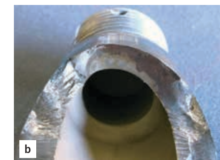
Figure 7: a) Fretting on the external surface of a taper shaft; b) A fatigue failure initiating from a taper shaft.
