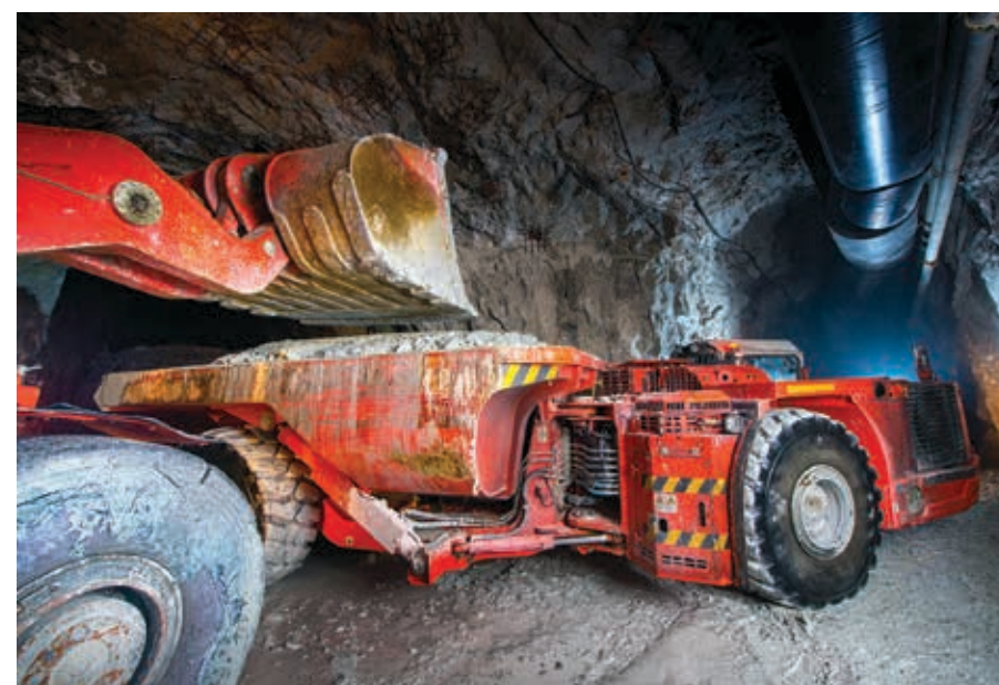
Frequently operated by remote control because of the hazards of falling rock in deep-level mining operations, underground downtime associated with repairs of load haul trucks can lead to significant production losses.
