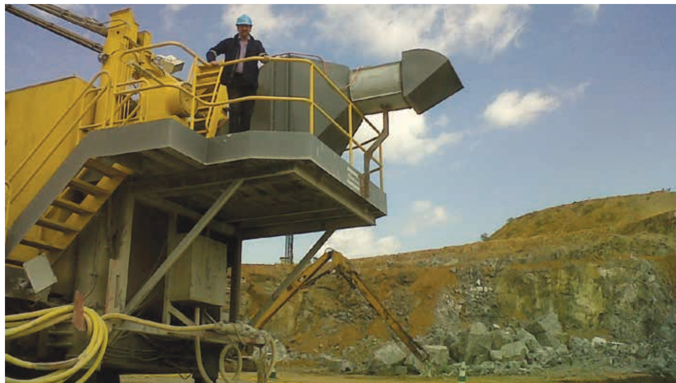
Attached to blast-hole drill-rigs, spin filters maintain the positive pressure inside the cabin preventing the ingress of dust very effectively.
