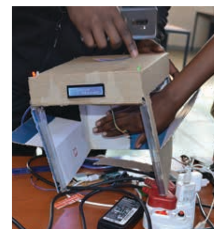
A team of Soshanguve engineering students in the Emerging Lab working on a mock-up loading cell (right) for their autonomous truck loading and blending system.
