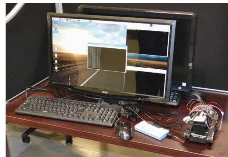
A model of the IIoT connected tracked mining vehicle to be used for the autonomous truck loading and blending system.
