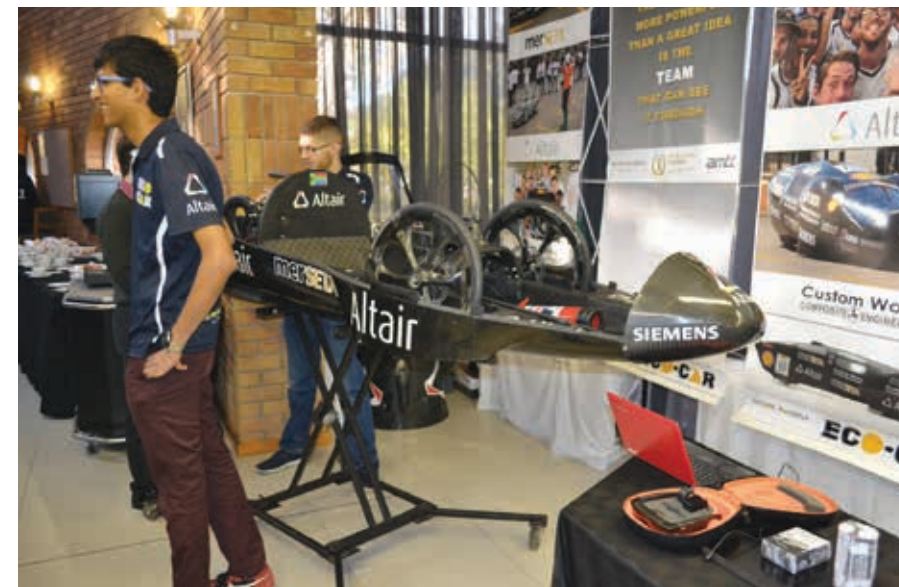
Nelson Mandela University's 2018 Eco Car, which incorporates new lightweight carbon fibre composite wheels, which were developed using Altair's HyperWorks design software with its OptiStruct topology optimisation solution.
