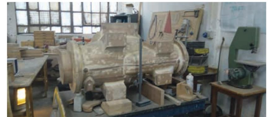
If required, APE Pumps also has the capability to make engineering design and pattern changes prior to casting.
