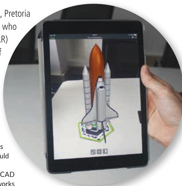
A 3D Solidworks model of a space shuttle published as an AR experience via Thingworks after associating the model with a licensed Thingmark.
