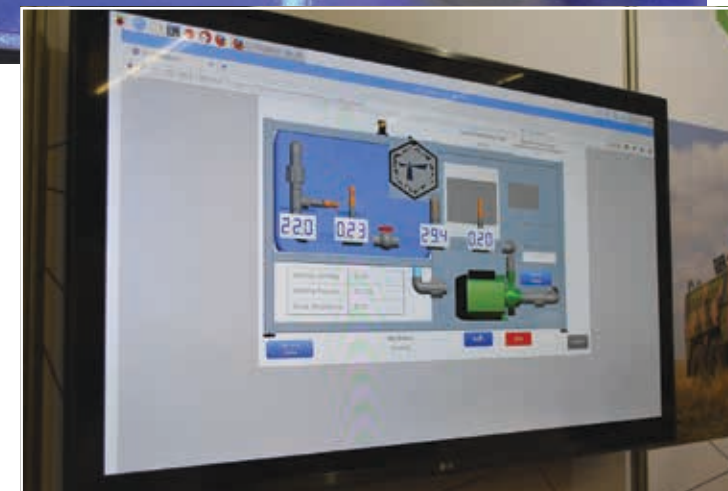
A pumping system and its associated AR experience being used for monitoring. As well as real time data measurements of the pump temperatures, pressures and flow rates, motor data can also be accessed along with external operating conditions such as the humidity, pressures and temperatures.
