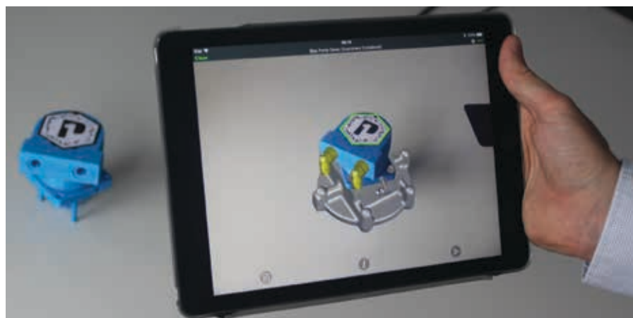
A second demonstration involving a hydraulic pump for a BobCat-type earthmover. After scanning the Thingmark and associating it to the pump, Anderson says that, unlike a QR code or bar code, a Thingmark aligns the pump with its surroundings and uniquely identifies position and scale information.
