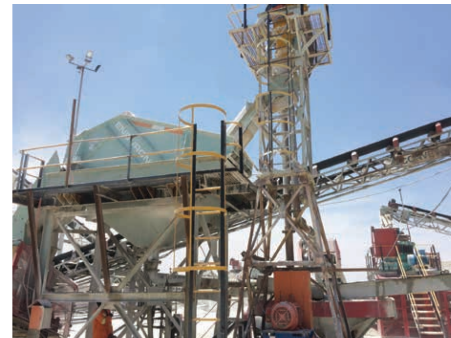
Above: Cavex 500CVX hydrocyclones discharging onto an Enduron dewatering screen.
