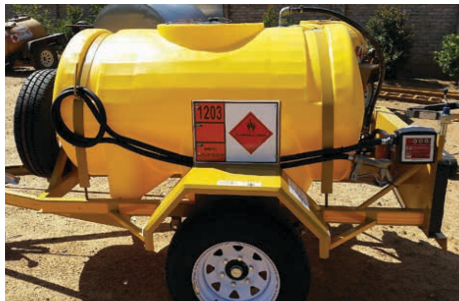
BMG's mobile filtration trailers provide reliable and cost-effective filtration of diesel, oils, lubricants and aviation fuel – not only at filling stations, but also on mines, construction sites and in the field.
