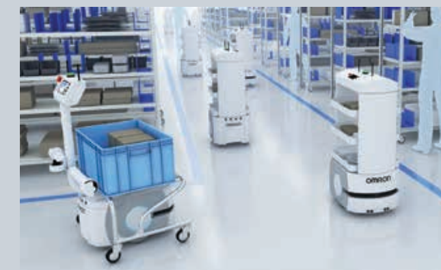
Omron AIVs can work in fleets of up to 100 mobile robots, and the workload is controlled by fleet management software.
