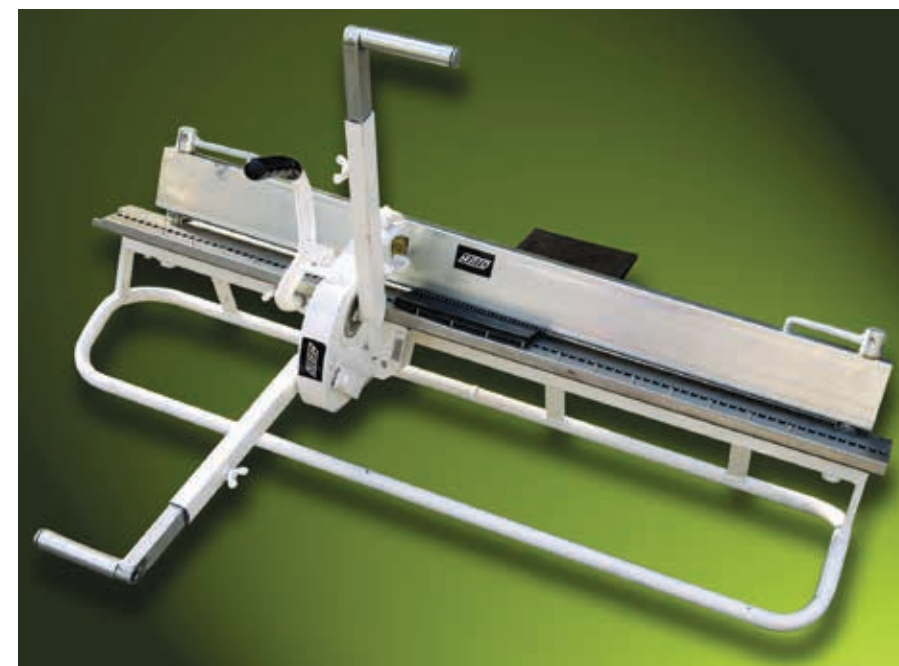
Mato's belt lacing system is an alternative to hot or cold vulcanisation for joining conveyor-belt sections.
