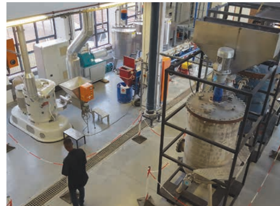
The chemical processing plant is equipped with high temperature and pressure chemical reactors, process tanks, a filter press, dryers and a bag house.
