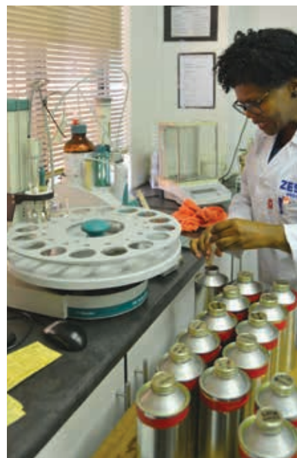
Oil samples loaded for automated processing and analysis by qualified WTA laboratory staff in WTA's state-of-the-art Heidelberg-based oil laboratory.
