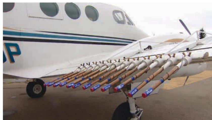
WAS is equipped with a Piper Cheyenne twin turbine aircraft fitted with a flare deployment system for cloud seeding.
