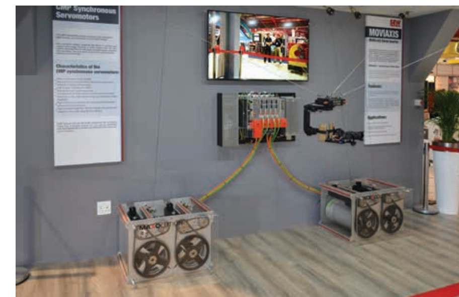
SEW-Eurodrive's MoviAxis servo inverter system was shown controlling a video camera via four pulley wheels reeling lines tethered to the top of the camera's support platform.
