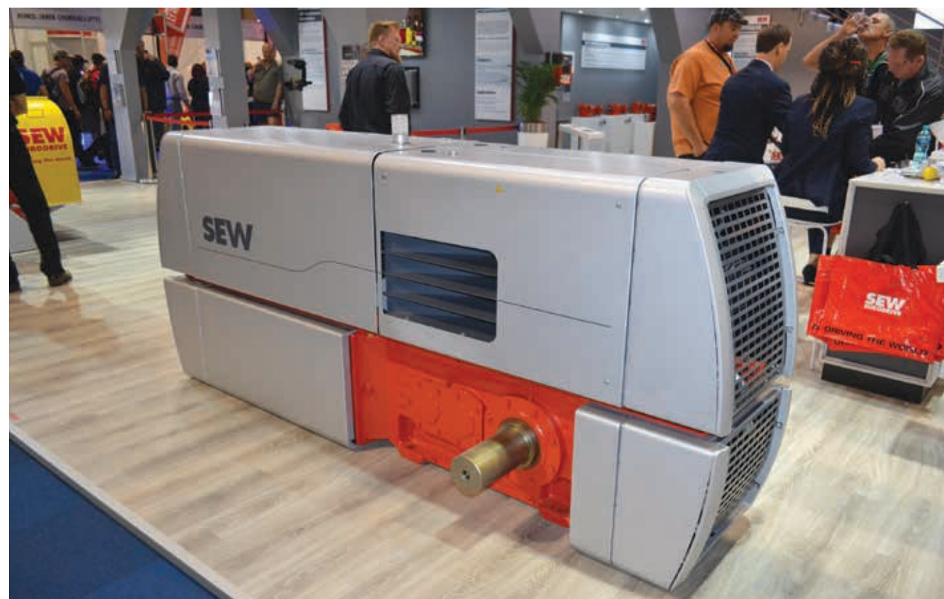
SEW-Eurodrive's MIG (mechatronic industrial gearbox) concept is an all in one compact power pack designed to be complete, efficient and very easy to assemble.
