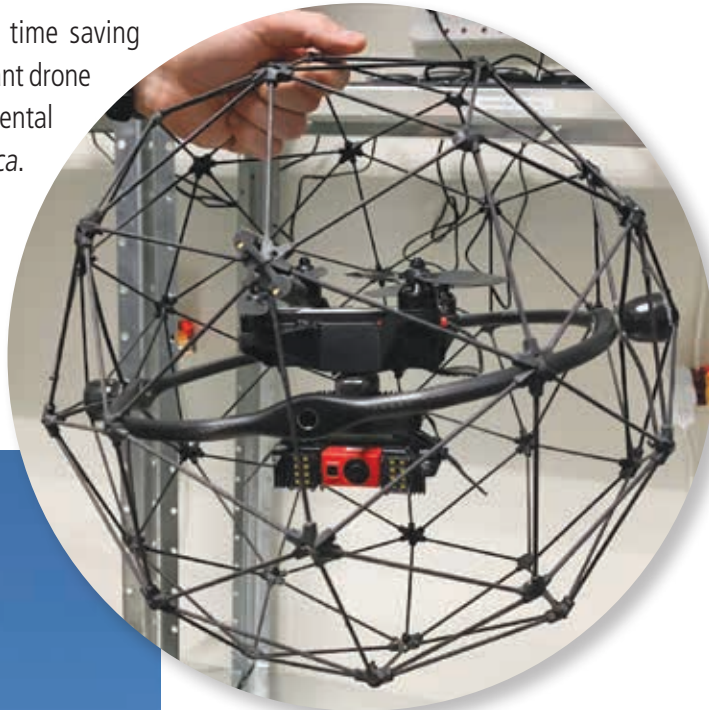
Skyriders Elios Sky Eye technology is the world's first collision-tolerant drone that can access controlled and confined spaces without any risk of crashing.
