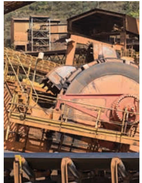
The use of Häggglunds direct drives on bucket wheel stacker/reclaimers enables avalanches to be overcome more easily. This has led to these drives being specified on all of Vale's new and retrofit bucket wheels.
