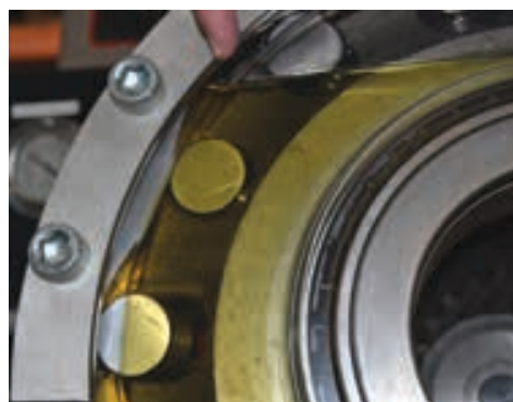
Häggglunds direct drive hydraulic motors have a fixed circumferential cam. Under hydraulic pressure, radial pistons with end rollers push against this cam causing the inner to rotate.
