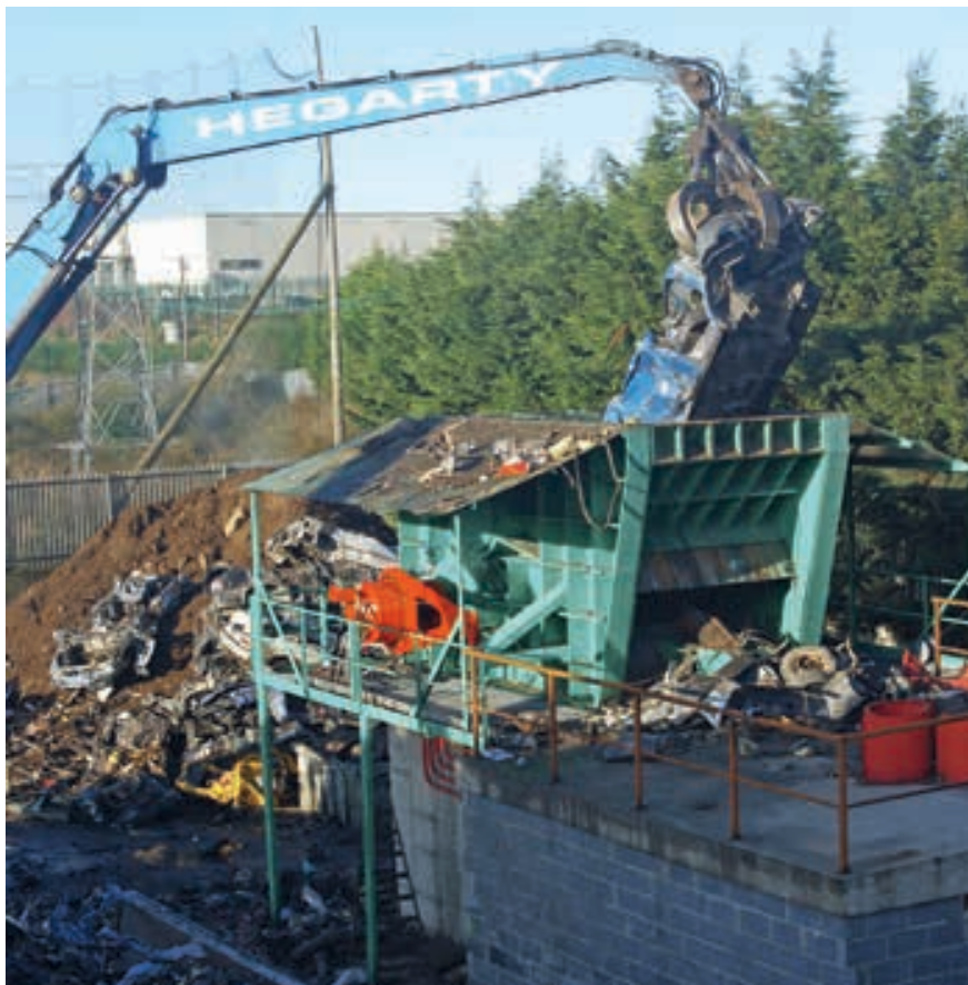
Spider's use on metal shredders in the recycling industry enables frequent knife jamming to be cleared by automatically and repeatedly reversing the knife blade when a stall is detected.
