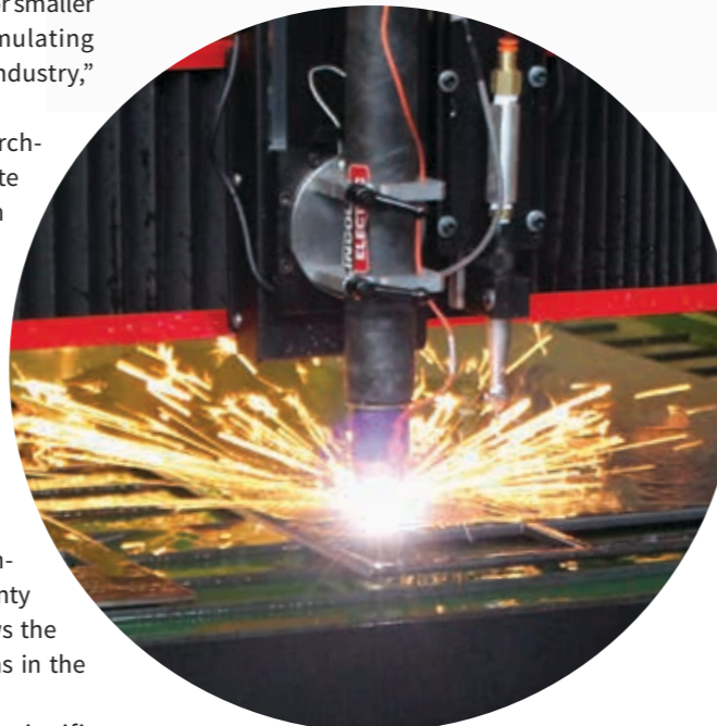
Lincoln Electric Torchmate 4400 and 4800 offer plate-cutting sizes of 1.25×1.25 m and 1.25×2.5 m, respectively and are entry-level systems that are ideal for light industrial applications.
