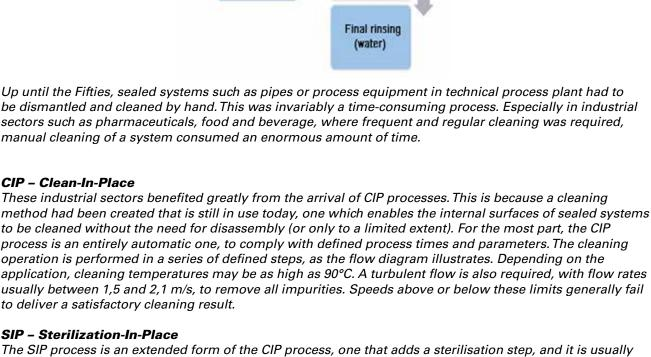
the actual CIP process. This ensures that any micro-organisms still active in the system are killed off with hot water or with saturated pure steam at high temperatures (typically 140°C). The effectiveness of this can be further enhanced by the addition of chemical disinfectants. Of course, WIKA offers appropriate measurement technology for CIP and SIP for a comprehensive range of measurement parameters.
