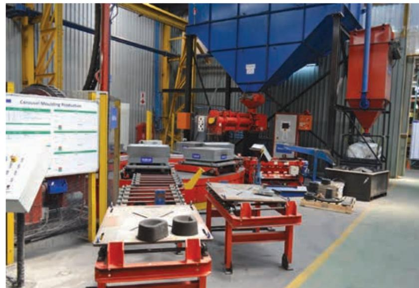
The carousel line at Isando uses a production-line process to prepare single or multi-cavity moulds to meet high-volume and high-variability needs.
