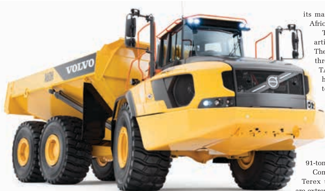
The payload of the A60H is 61 short tons or 55 metric tons (tonnes).
