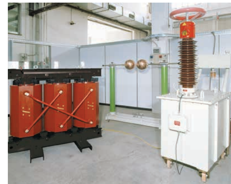
Cast-resin transformers in the test bay.
