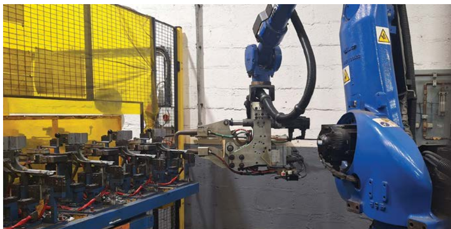
Yaskawa's servo-driven spot welding actuators are mounted onto the end of the robot arm, and they fully integrate into the robot as a seventh control axis.
