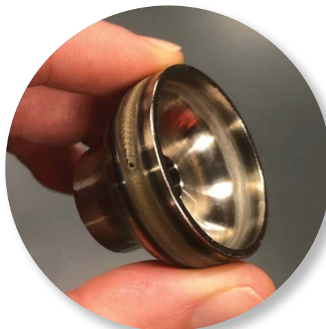
Factories producing high purity ingredients must ensure that the inside surface of every connecting tube is perfectly flush and smooth.
