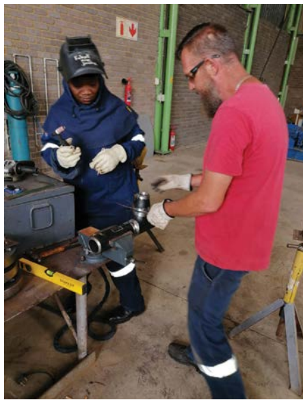
Left: Setting up a precision piping component and, right: the weldment prepared for TIG/GTAW welding.
