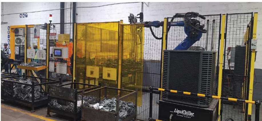
The latest collaboration project between D&L Engineering Solutions and Yaskawa Southern Africa is a component production line for the assembly of a safety critical automotive component.
