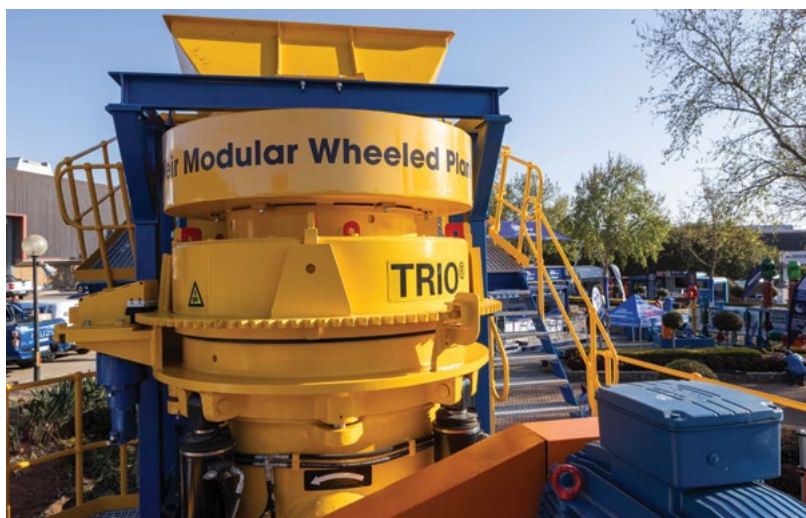
The WMWP features a TRIO TC 36 cone crusher designed for secondary and tertiary crushing.
