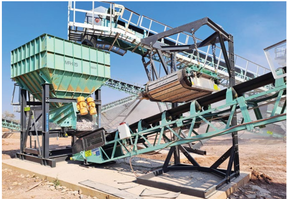
The Pilot Modular Feed Hopper MFH25 is used to control the feed to the cone crusher and an MPM910 magnet is used to remove tramp metal before the cone crusher.
