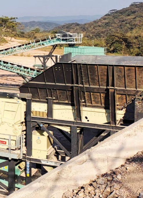
The Pilot Modular Feed Hopper MFH25 is used to control the feed to the cone crusher and an MPM910 magnet is used to remove tramp metal before the cone crusher.
